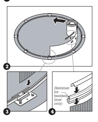
e. Work around the foundation until the entire pool wall is uncoiled into the bottom rails and the top edge is covered with slotted tubes and connectors (and beaded liner retainers if you have a beaded pool liner).
