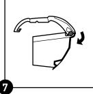
upper half (key 9). Tip lower half of the top connector (key 10) into place (the upper half of the top connector will rotate on the corners of the lower half like a hinge, locking the two parts together).
