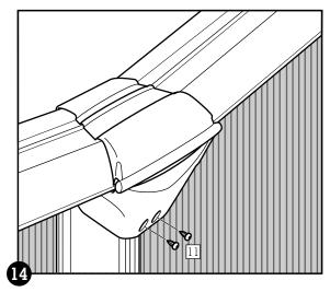
g. For oval pools only: at the transition points only, where the end rail meets the side rail, make sure the side rail lines up properly with the end rail. If it doesn't line up the connector will appear crooked from above (see diagram 15). If the connector isn't centred between the rails, temporarily remove the
