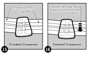
connector and loosen the screws on the side rail. Shift the side rail in or out from the centre of the pool until the connector can be properly centred between the rails (see diagram 16).
