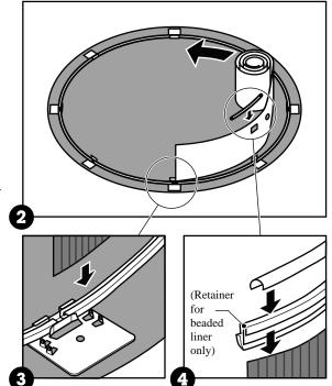
e. Work around the foundation until the entire pool wall is uncoiled into the bottom rails and the top edge is covered with slotted tubes and connectors (and beaded liner retainers if you have a beaded pool liner).
