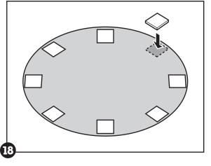
d. The patio stones **must** be sunk into the ground so the tops are flush with the soil around them. Use the carpenter's level to make sure the patio stones are perfectly level and flush with the ground. Use the carpenter's level and a 2-by-4 between patio stones to make sure the stones are level with each other.
