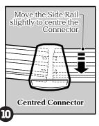
connector and loosen the screws on the side rail. Shift the side rail in or out from the centre of the pool until the connector can be properly centred between the rails (see diagram 10).
