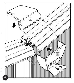
e. Open the door on the outer half of the top connector. Line up the two screw holes with the two holes in the vertical column. Fasten them together with two self-tapping screws (key 11). Tighten the screws and close the door.
