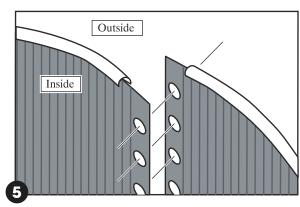
b. To line up the holes, make the circle bigger or smaller by nudging the base plates in or out with your foot.
